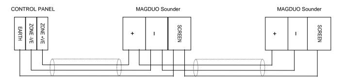
The MAGDUO Sounder can be mixed on the same zone as other types of MAGDUO devices. The above diagram shows how to make the zone positive, zone negative and screen connections between the control panel and MAGDUO Sounders. Refer to the instruction leaflets supplied with other MAGDUO devices for their equivalent wiring/terminal labelling details.
